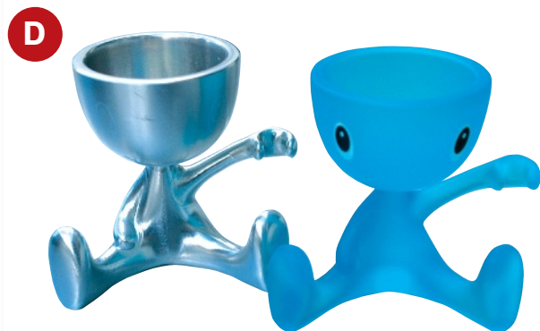
Using Open Mind's HyperMill software to simulate the milling sequence of an egg holder (A, B, C); the resulting prototypes were milled in the DMU 60 monoBLOCK milling machine (D).
