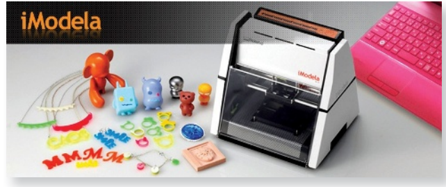
Roland DGA's iModela, a hobbyist's milling machine, is available for less than $1,000.
